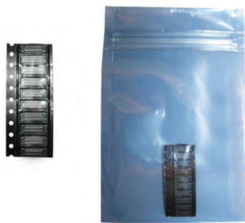
Place Connectors into Reel
